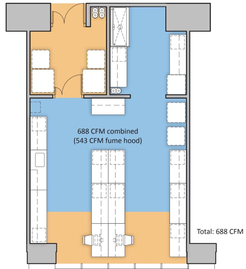
*An unenclosed support room can accommodate the 6' 543 CFM hood without the additional air and energy premium*
