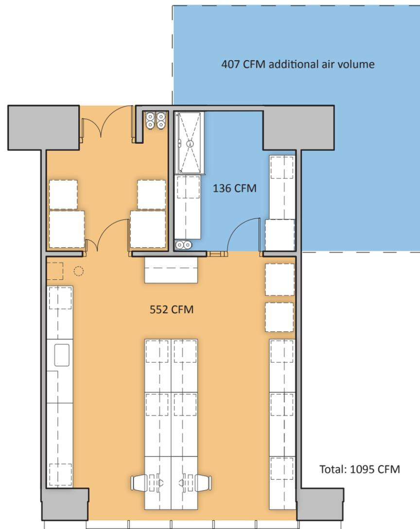
*A 6' fume hood consuming 543 CFM in an enclosed support room exceeds the minimum exhaust air requirement and additional air volume is required*
