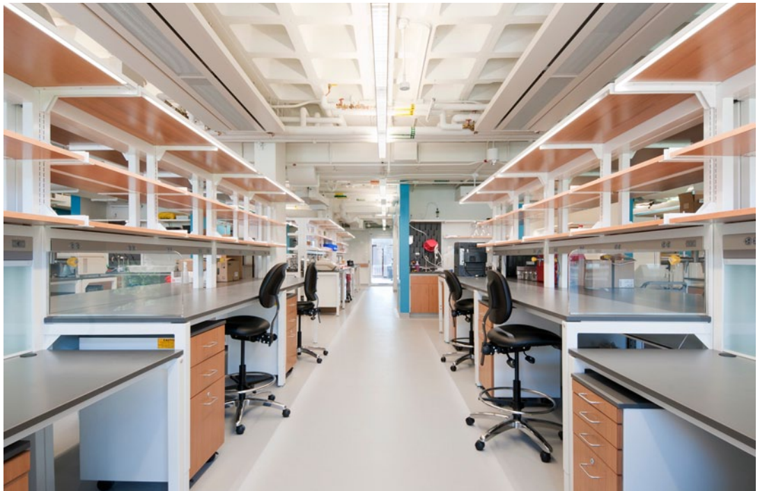
Harvard University, Sherman Fairchild Center for Stem Cell and Regenerative Biology: The laboratory developed a novel approach to reducing the energy profile by utilizing LED lighting and chilled beams for supplemental cooling. LEED-CI 3 Platinum Certified with the highest number of LEED-CI points (95) achieved by any LEED-CI lab in the world to date.
